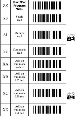
**Single Read** - When a bar code has been decoded, the reader will be turned OFF. The reader must be triggered again to read another label. This option and "Disable trigger" cannot be programmed at the same time.
